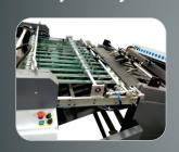
Sheet Ejection mechanism Non-stop delivery Pneumatic operations
